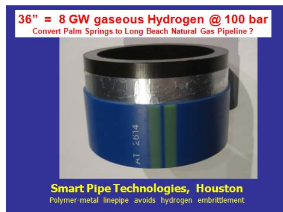
Figure 4. Polymer-metal hybrid linepipe for GH 2 . Thin Al or Cu foil H 2 perm barrier. Sample by Smart Pipe, Houston. Not tested for GH 2 service: ORNL origin; more R&D required.
