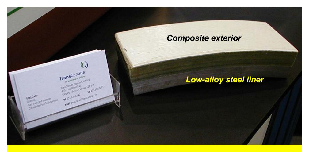
Composite – Reinforced Line Pipe (CRLP) 3,400 psi, .75" X70 steel plus .75" composite
