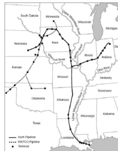
Fig. 9. Extant liquid NH 3 pipeline and storage terminal network, handling ~15 MMT per year, primarily for N-fertilizer, of which ~60% is imported.
