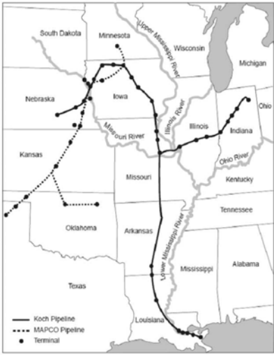
Fig. 13. Extant USA liquid NH 3 pipeline and storage terminal network, handling ~12 MMT per year, primarily for N-fertilizer, of which ~60% is imported.
