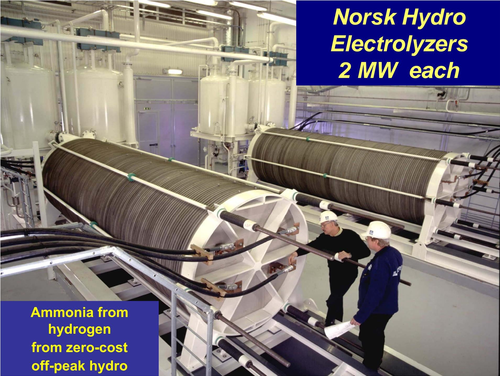
A photograph of a large industrial facility containing several massive electrolyzers. The electrolyzers are large, cylindrical units with a complex internal structure, mounted on a metal frame. In the background, there are several large white storage tanks and a network of pipes. Two workers in white hard hats and dark clothing are standing on a platform in the foreground, looking at a set of plans. The overall environment is clean and well-lit.
