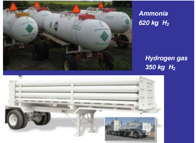
Figure 3. Energy storage: (top) Agricultural fertilizer liquid \text{NH}_3 “nurse tank”: capacity 1,450 gallons @ 265 psi = 620 kg hydrogen each. Capital cost ~ $9.5K each. (bottom) Gaseous hydrogen tube trailer: capacity 5,800 gallons @ 3,200 psi = 350 kg hydrogen. Capital cost ~ $750K
