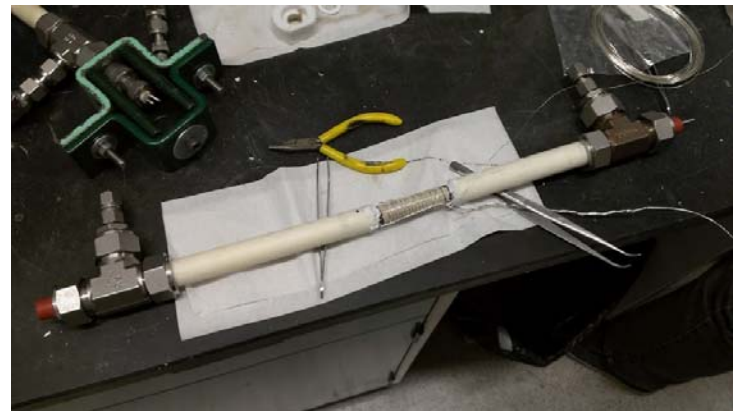
Figure 11. Proton conducting ceramic (PCC) tube section (center) installed between alumina fixture tube sections for solid state ammonia synthesis (SSAS) test
