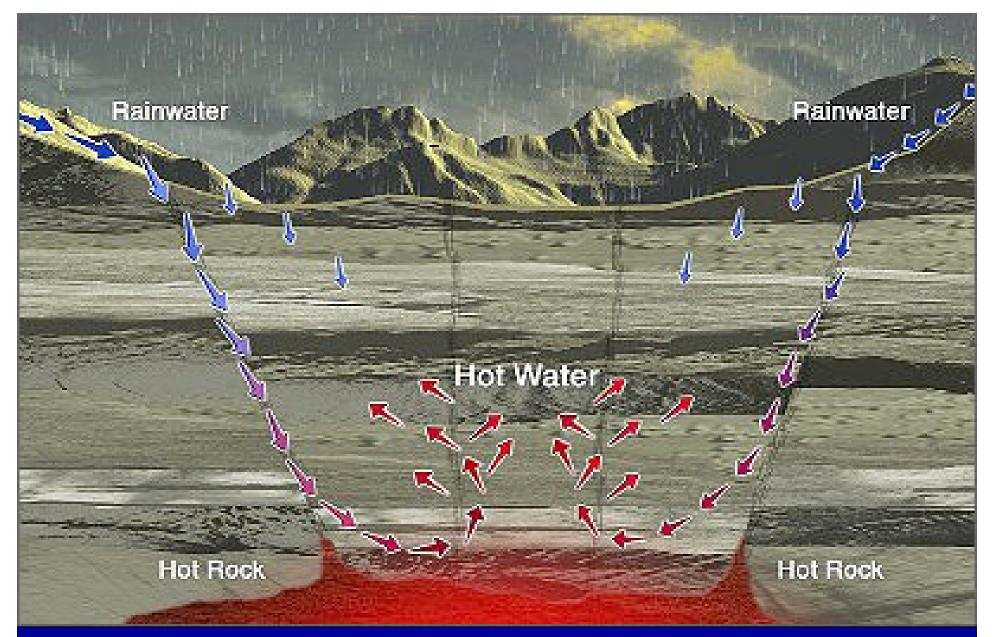
Geothermal: hot water, surface recharge
