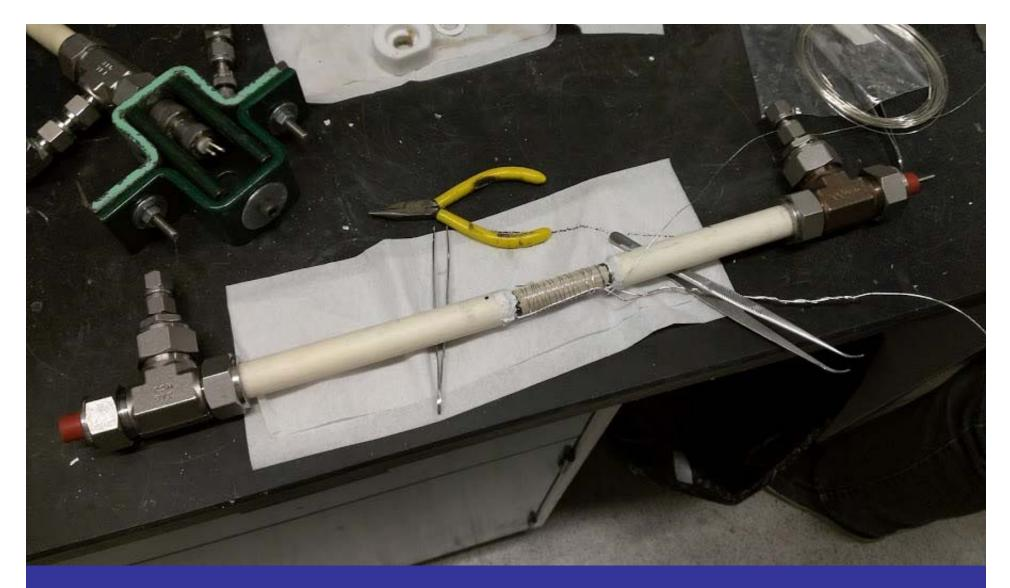
Center: PCC tube 33 cm<sup>2</sup> active area. Current collectors installed. Sealed to alumina support tubes. Setup is leak-free.
