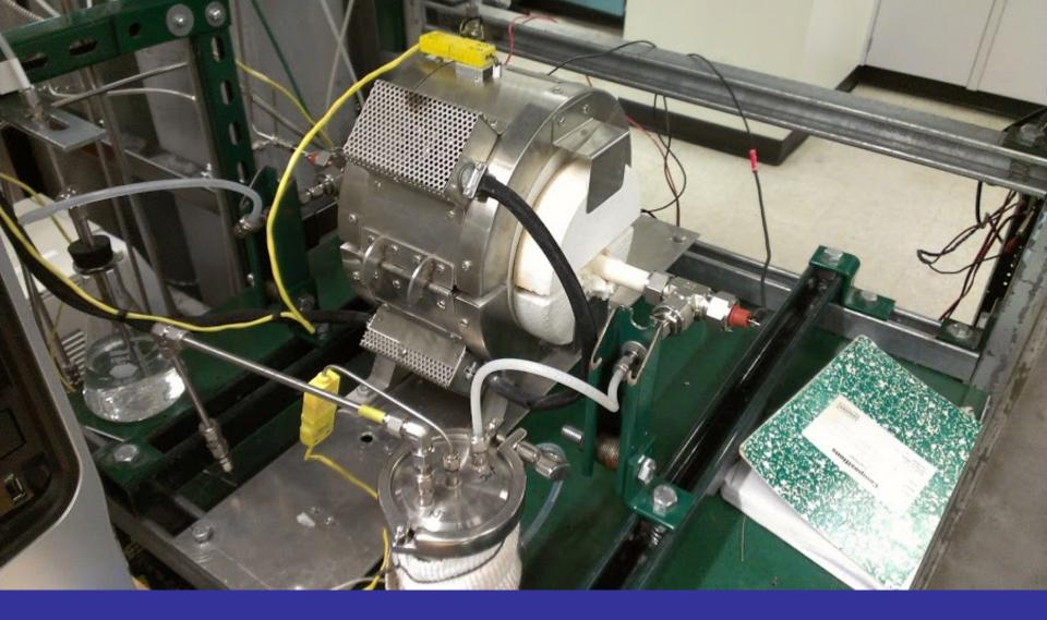
Tube assembly installed in test fixture.
