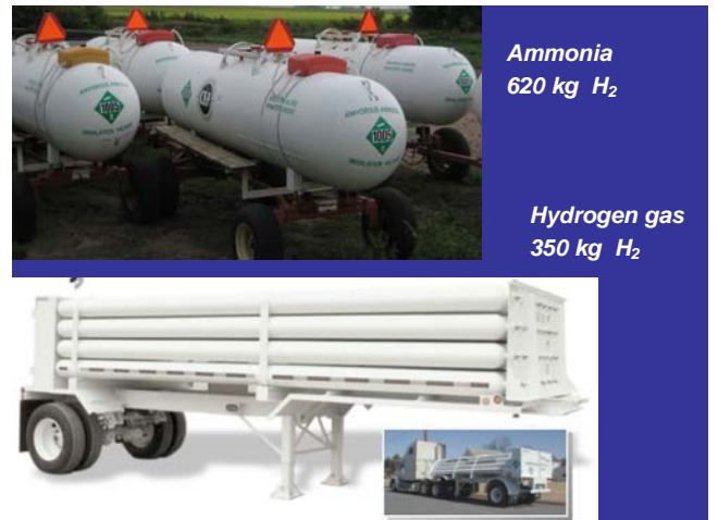
Figure 3. Energy storage: (top) Agricultural fertilizer liquid NH 3 “nurse tank”: capacity 1,450 gallons @ 265 psi = 620 kg hydrogen each. Capital cost ~ $9.5K each. (bottom) Gaseous hydrogen tube trailer: capacity 5,800 gallons @ 3,200 psi = 350 kg hydrogen. Capital cost ~ $750K
