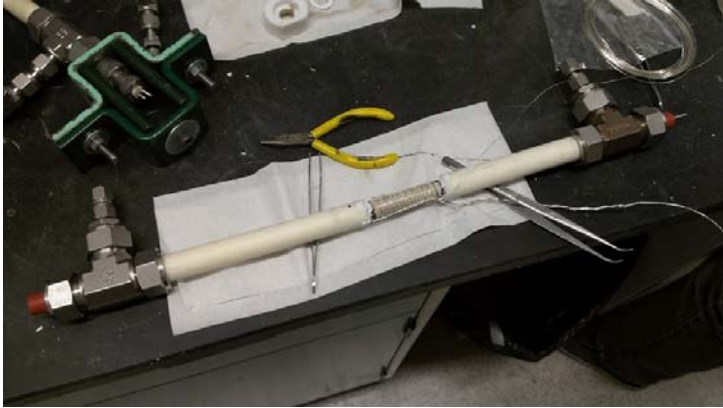
Figure 11. Proton conducting ceramic (PCC) tube section (center) installed between alumina fixture tube sections for solid state ammonia synthesis (SSAS) testing.
