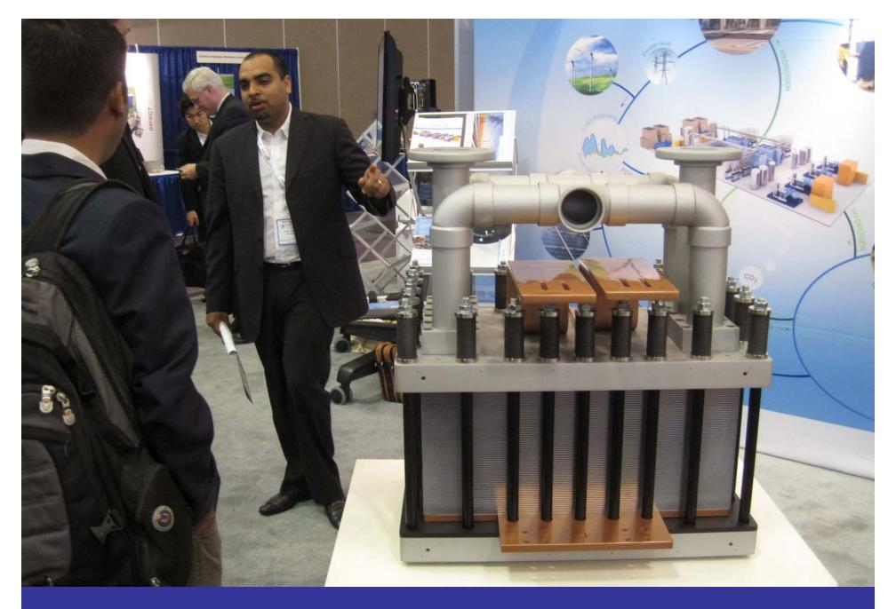
Hydrogenics 1 MW PEM Electrolyzer, June 2013
