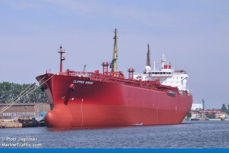
Clipper Sirius 54,000 DWT LPG or NH3 tanker Fully refrigerated
