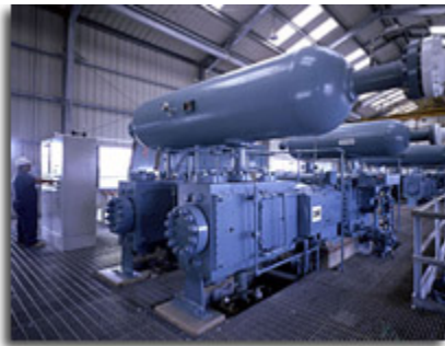
Three 8500 horsepower HHE-VL units compress natural gas to 2700 psi into underground storage caverns.
