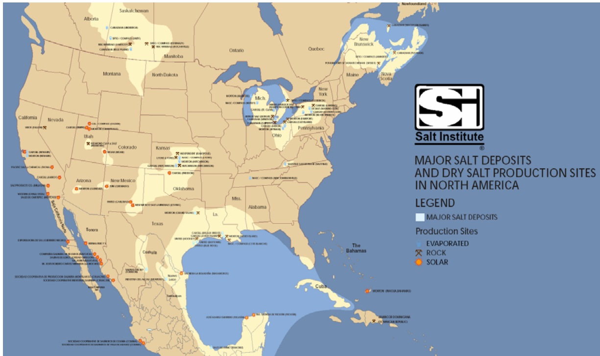
Figure 29. Large underground dry salt formations which may be suitable for solution mining, to create large GH 2 storage caverns.
