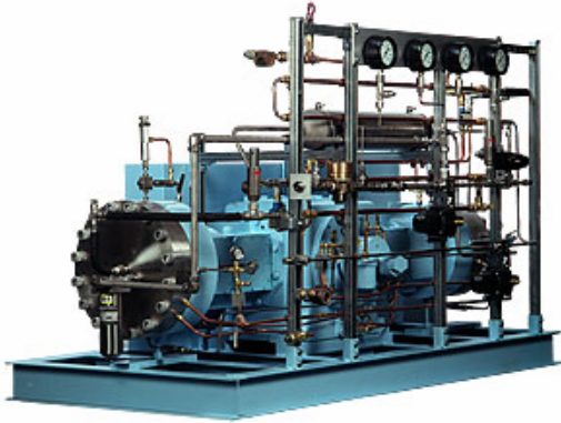
Figure 9. A large diaphragm compressor by PDC Machines.
