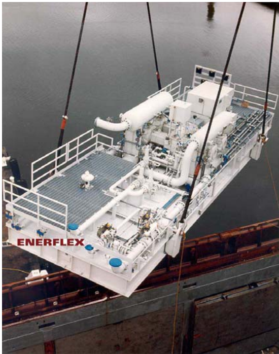
Figure 10. A large reciprocating compressor, NG service; 3,000 hp electric motor drive.
